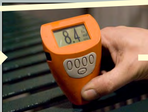
Inspect to 8 mil Average Thickness (30 mil for EcoSoft)
