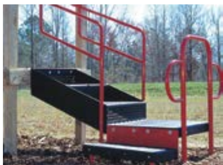
ADA Transfer Station —Handrails included. Punched steel with matte brown PVC finish. For 30" to 36" deck heights
