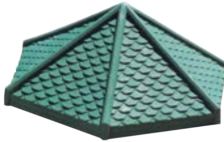
Hexagon 07699—One-piece roto-molded double wall construction. 94" flat-to-flat; 111" point-to-point; 44" tall
