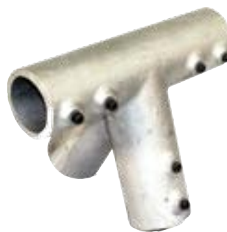
Middle Frame Fitting FF-02 —Heavy duty two legged middle frame fitting with 2 3/8" legs. These are for schedule forty 2" pipe. Available as uncoated only
