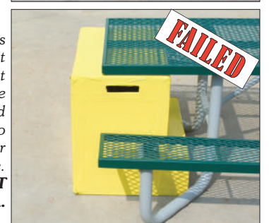
The manufacturer of this table claims “universal access” but notice that the ADA Clearance Box does not fit completely under the top. The frames get in the way of the required 5” x 9” x 30” toe clearance space, so it does not provide total wheelchair access under the table.
