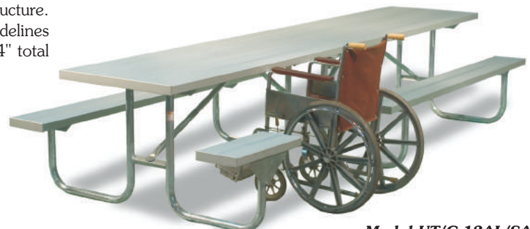
Model UT/G-12AL/SA 1-5/8" OD galvanized frames, 12 ft., clear anodized aluminum, two side access openings for two wheelchairs.
