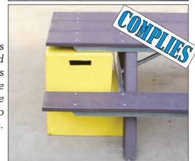
Pilot Rock AT Series A-frame tables are available with a top extended one foot at each end. This provides adequate knee clearance under the table top, and the A-frame space provides the toe clearance needed to meet the guidelines.
