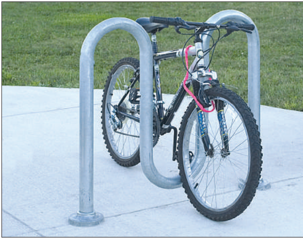
Model SRP/G-5 bike rack, surface mount installation with base plate, includes cover caps, will park up to 5 bikes.
