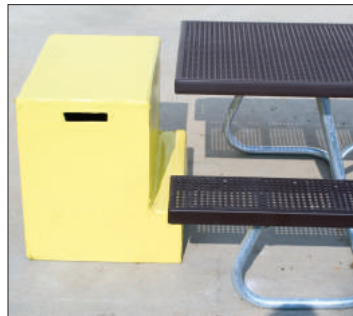
The ADA Clearance Box built to the required dimensions, including knee and toe clearances, approaches a Pilot Rock W Series Universal Access picnic table.
