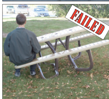
This table brand does provide enough knee and toe clearance under the top to meet ADA guidelines. But the inadequate frame design (less than transverse frame angle bends) and the light weight materials used to construct the frames and top/seats create instabilities in this table which make it a problem for the public to use safely.
